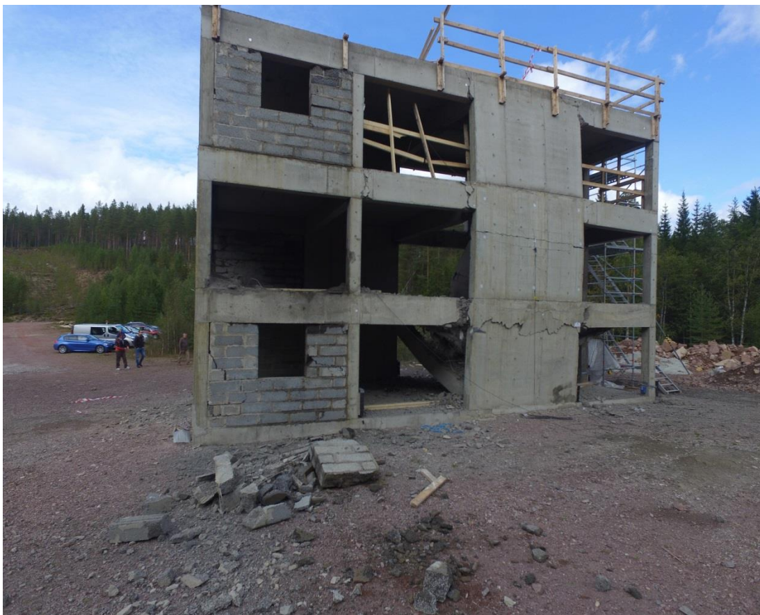
Pilot building's condition after internal blast (floor collapsed and external walls/columns were severely displaced)
