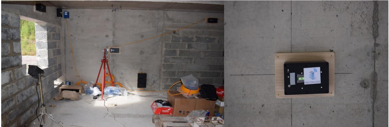
Set up of data hubs, temperature sensors and accelerometers at ground floor (left) & the positioning tag at the mid-span of a wall (right)
